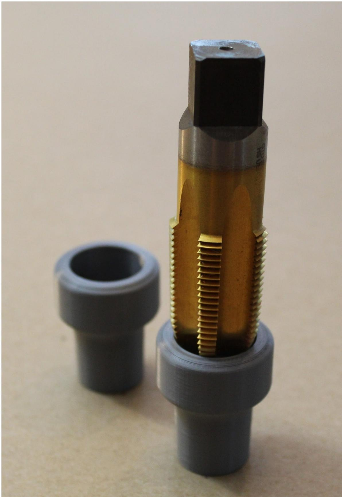
Last, we will tap the adapter to the pressure sampling lines.
