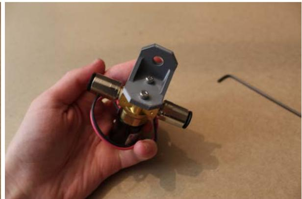
**Step 2. Attach the pressure relief valve to its adapters.**
