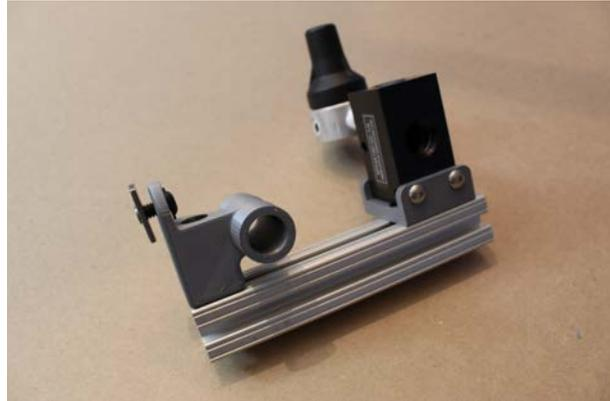
**Step 6. Attach corner brackets to finish this frame piece.**
