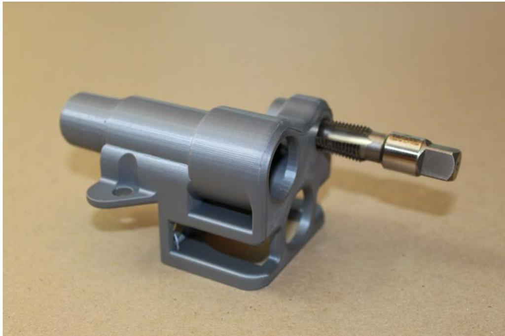
**Step 2.** Use the M16 tap to thread the hole on the opposite side of the Sensor Atrium, where the oxygen sensor will attach.
