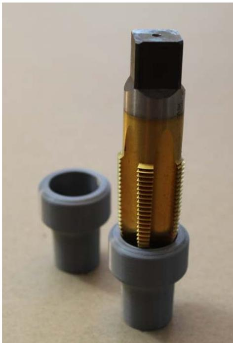
Last, we will tap the adapter to the pressure sampling lines.
