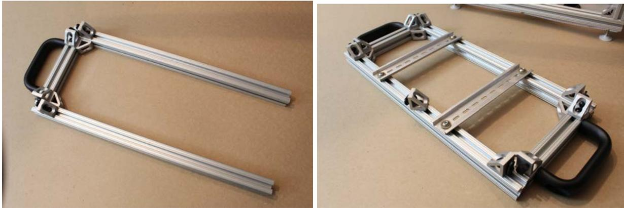
**Step 6. Finally, slide the top frame directly into the vertical 80/20 channels of the device, and tighten all hex screws.**
