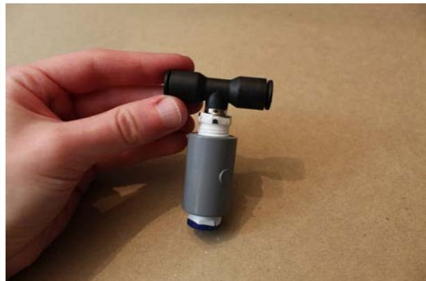
**Step 3. Attach the luer lock connectors to the luer lock filter mount.**
