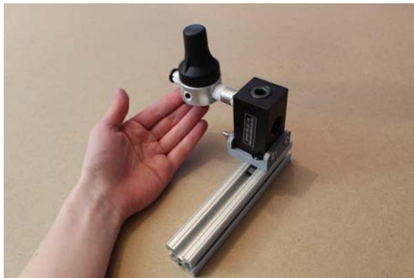
**Step 5. Attach the “Expiratory outlet bracket to PEEP”.**
