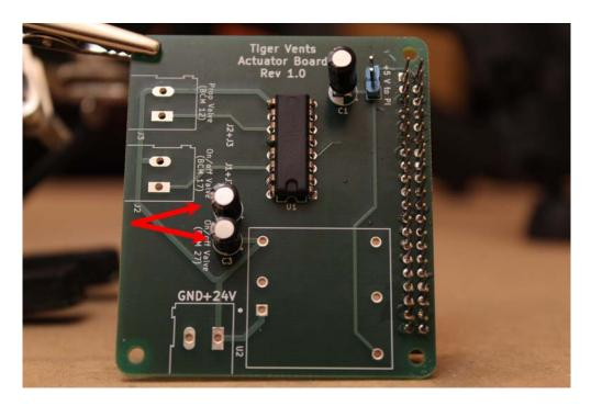
Step 6. Solder the 24-to-5 V DC-DC converter (CUI PDQ15-Q24-S5-D) onto the board, as shown.
