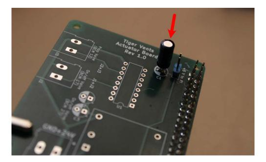
**Step 4. Solder the ULN2003A (Darlington array) into place (position U1).** Be sure to match the notched end of the part to the notch indicated on the board.
