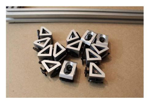
Step 3. Attach gusset (corner) brackets, as shown.
