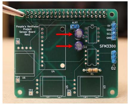
Step 5. Solder the TL7660 (the rail splitter for the INA126) onto the board (position U1). Be sure to orient the small circle on the top of the part to the indicated notch drawn on the board.
