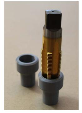
Last, we will tap the adapter to the pressure sampling lines.
