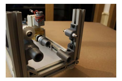
Step 8. Attach the third vertical 80/20 leg, then attach the proportional valve mount. Insert a third, short  $(5 \frac{7}{6})$  80/20 piece, then tighten the hex screw to hold it in place. Use another standard hex screw/nut to attach the proportional valve mount to this piece, towards the inside of the device, such that the push-to-connects roughly align vertically with the push-to-connect on the sensor atrium.
