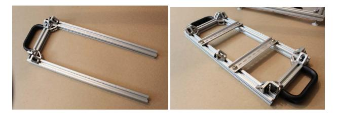
Step 6. Finally, slide the top frame directly into the vertical 80/20 channels of the device, and tighten all hex screws.
